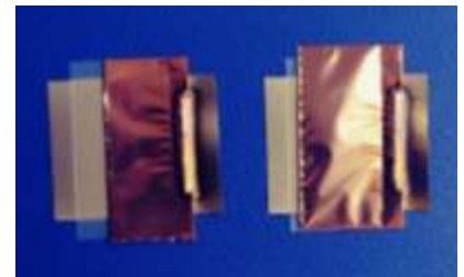
Figure 3. Cu Foil Welded to Ni-coated Cu Tab
