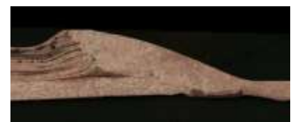
Figure 4. Cross section of Cu Foil Weld
