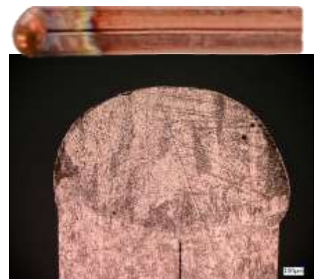
Figure 3. Top Image highlights the uniform spherical shape and heat affected zone generated from the process. Bottom image is a cross section showing no porosity or defect within the welded area.
